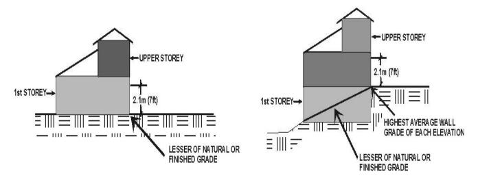
"veranda" for a single family residential building or coach house means a one storey high roofed portico, gallery or porch adjoining an exterior wall or walls of a building and open at all other sides with the exception of necessary structural support columns and a guard or rail not exceeding a height of 1.1m (3.5 ft.) and with a floor not higher than the lowest above-grade building floor on the side of the building to which it is attached;
