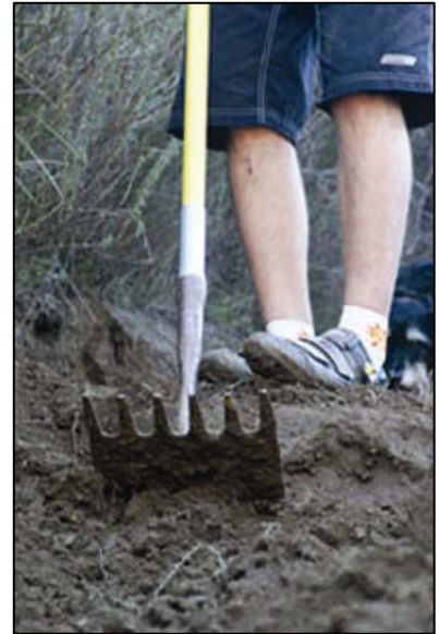
Figure 18: The McLeod is a multipurpose tool that acts as a rake, blade and tamper.
