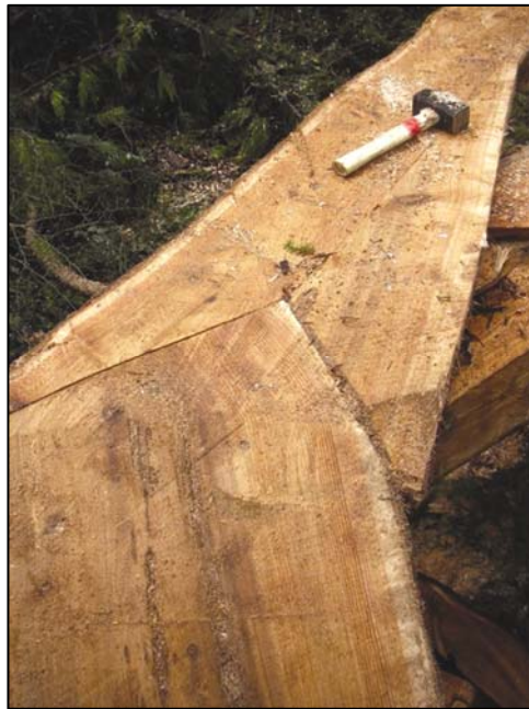
Large pieces of wood and minimal fasteners increase the longevity of structures.
