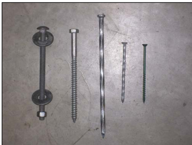
Recommended fasteners: (left to right) galvanized lag bolt, galvanized lag screw, ardox spike, ardox nail, deck screw.
