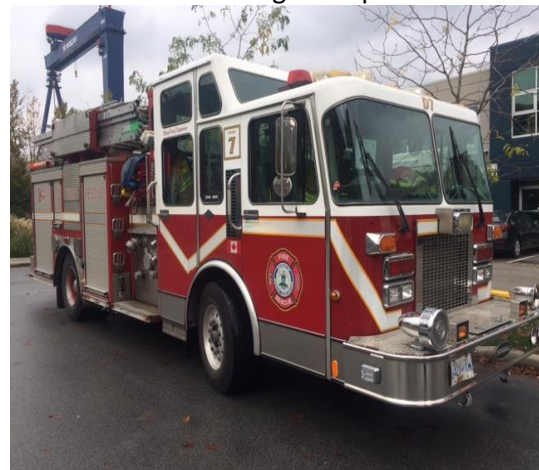
DE7 – 1994 Spartan Superior Pumper Engine, 203350 Km, 300 Gallon Tank Capacity, Two Stage Pump
