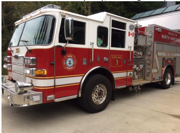
DE3 – 2016 Pierce Pumper Engine, 53346 Km 344 Gallon Tank Capacity, Two Stage Pump
