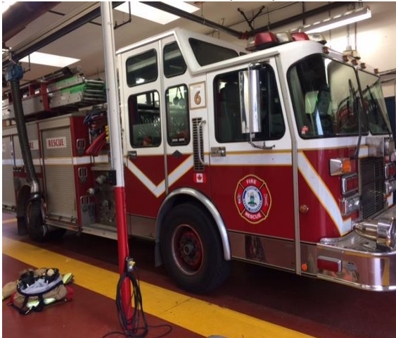
DE6 – 1997 Spartan Superior Pumper Engine, 18898 Km, 300 Gallon Tank Capacity, Two Stage Pump
