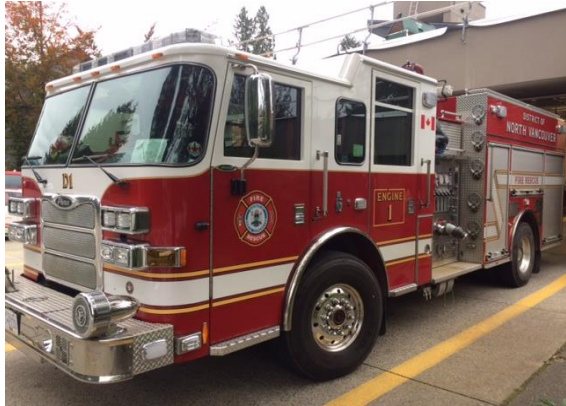
DE1 – 2014 Pierce Pumper Engine, 68545 Km 300 Gallon Tank Capacity, Single Stage Pump
