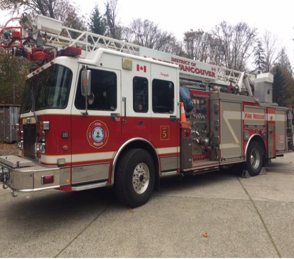
DQ5 – 2003 Spartan Smeal Quint, 148857 Km 300 Gallon Tank Capacity, Single Stage Pump, 55' Ladder
