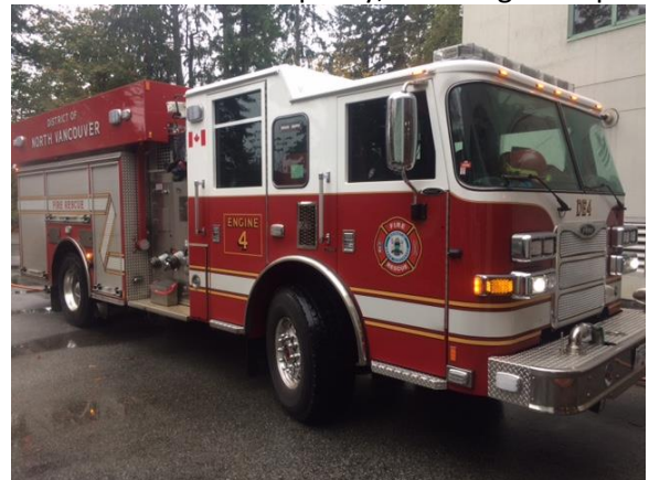
DE4 – 2016 Pierce Pumper Engine, 42750 Km 336 Gallon Tank Capacity, Two Stage Pump
