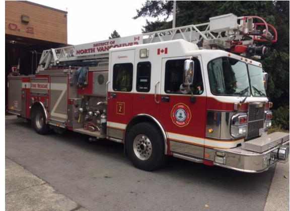
DQ2 – 2006 Spartan Smeal Quint, 107321 Km 300 Tank Capacity, Single Stage Pump, 55' Ladder
